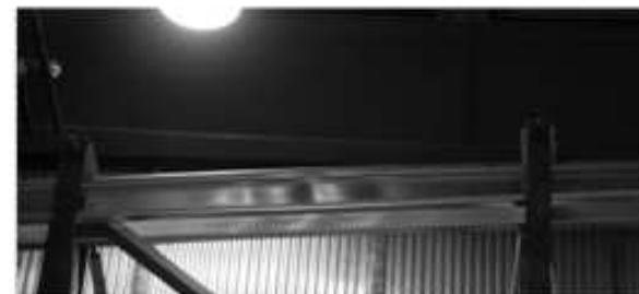
Figure 6: Elastic local buckling (left) and failure in the compression chord (right) in test 5
