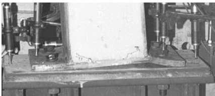
b) plate-failure (specimen CCB2)
