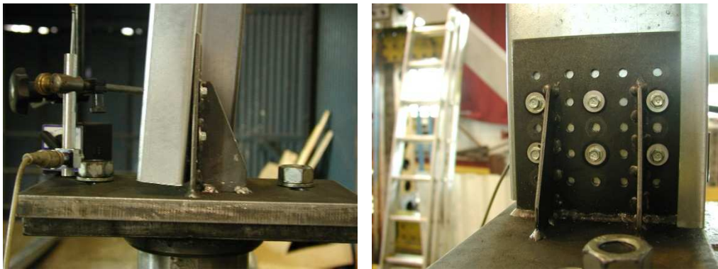
Figure 4. Load introduction: gusset plate and self-drilling screws
