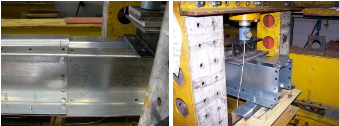
Figure 40. Test arrangements: reinforced section at the end of overlap and end support tests
