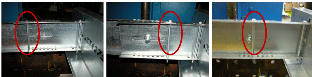
Figure 67. Bolt positions 1, 2 and 3 in the adjustable piece tests
