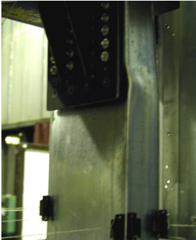
Figure 48.: Plastic mechanism at the load introduction (SimpleC, C01).
