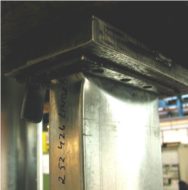
Figure 50.: Plastic mechanism at the load introduction (CompressionC, C05).
