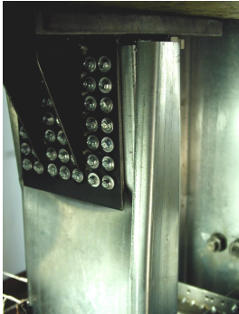
Figure 49.: Plastic mechanism at the load introduction (DoubleC, C09).
