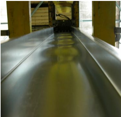
Figure 26.: Local buckling in the web.
