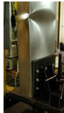
Figure 47.: Failure of specimen.
