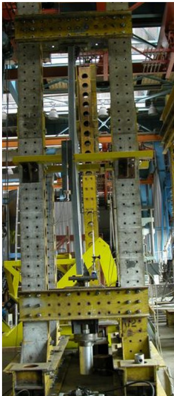
Figure 2.: The loading frame.
