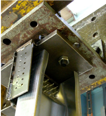
Figure 51.: Plastic mechanism at load introduction (short screw layout, C68).
