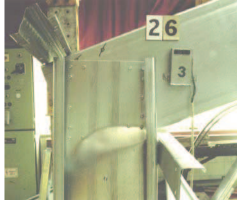
Figure 2.24: Buckling in the column.
