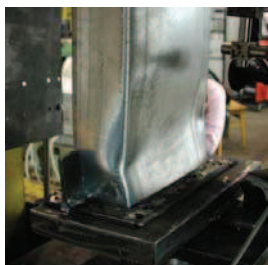
(a) end crushing
