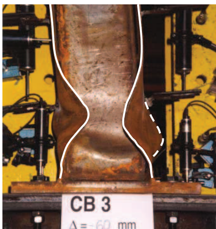
Figure 3.7: Plate buckling patterns; steel and composite specimens.
