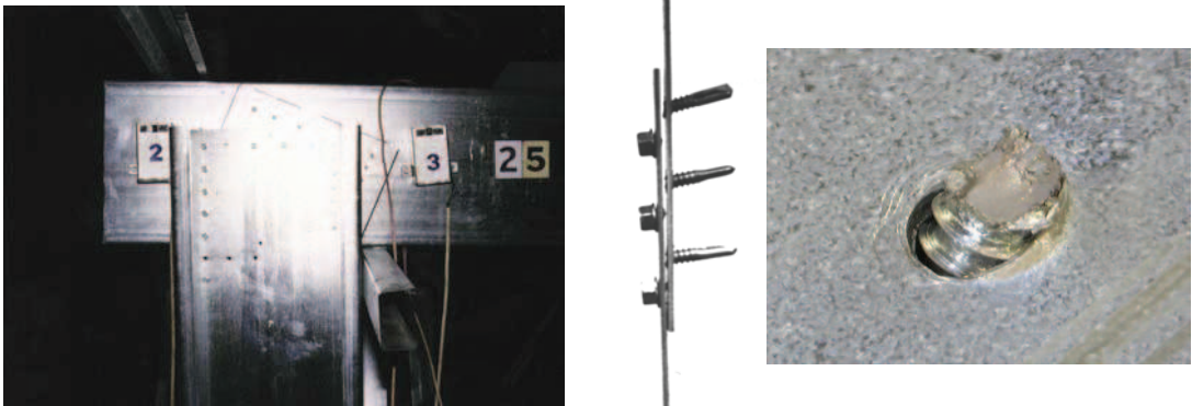
Figure 2.20: Illustration of shearing failures.
