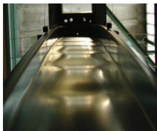
(b) plate and flexural buckling
